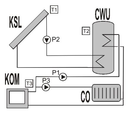
Fig.1 Operation layout of the regulator
